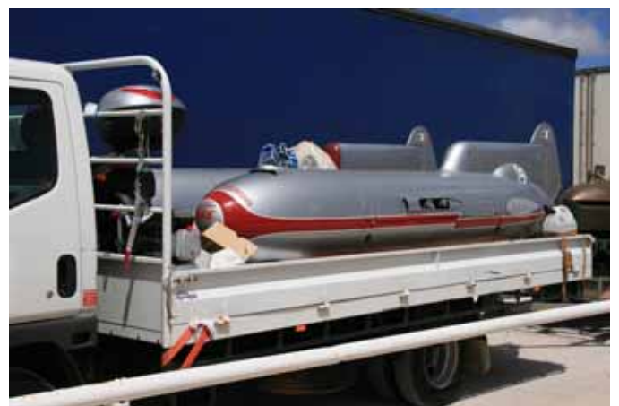
Twin bodied special, driver sits in one pod, motor in the other.
