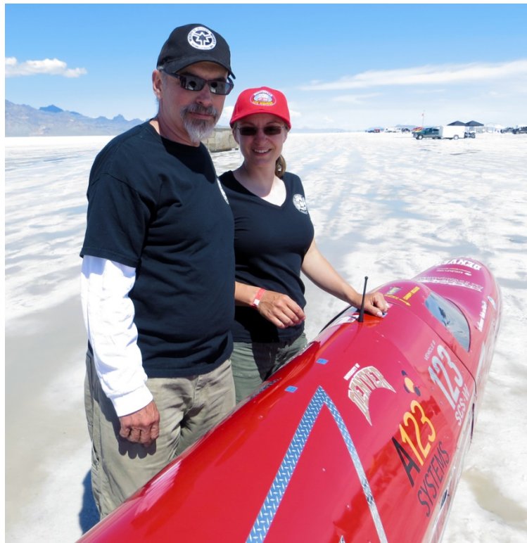
The two small pieces of blue tape right above the University of Denver logo mark the Centre of Gravity (CG) and the Centre of Pressure (CP) of the KillaJoule. The CG is in front of the CP, just as it should be. Marking them with tape made the technical inspectors quite happy.
