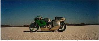
The bikes wheelbase has been lengthened to the maximum permissible for it's class and the front forks raked slightly to produce slower steering.
