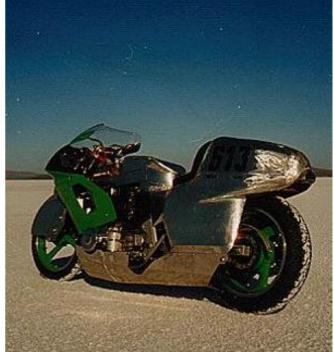
The bike is a modified 1981 Kawasaki Z1000 J Class: MPS 1000 (Modified, Partial Streamlining, 1000cc) Highest speed recorded - 157 MPH March 2000 The motor produces approx. 100HP and remains relatively stock.
